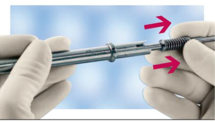
**VI** Pull inner tube out of outer shaft.
